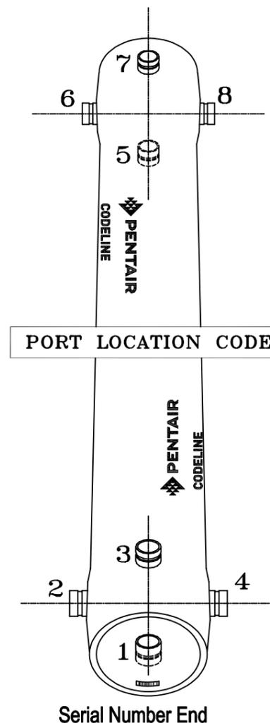
CODELINE BODY LABELS ARE PLACED AT 90° ON SERIAL NUMBER END AND AT 270° ON THE OPPOSITE SIDE END
